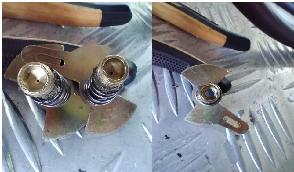
Figure 27: Modification of gas nozzle size for biogas (left before and right after)
