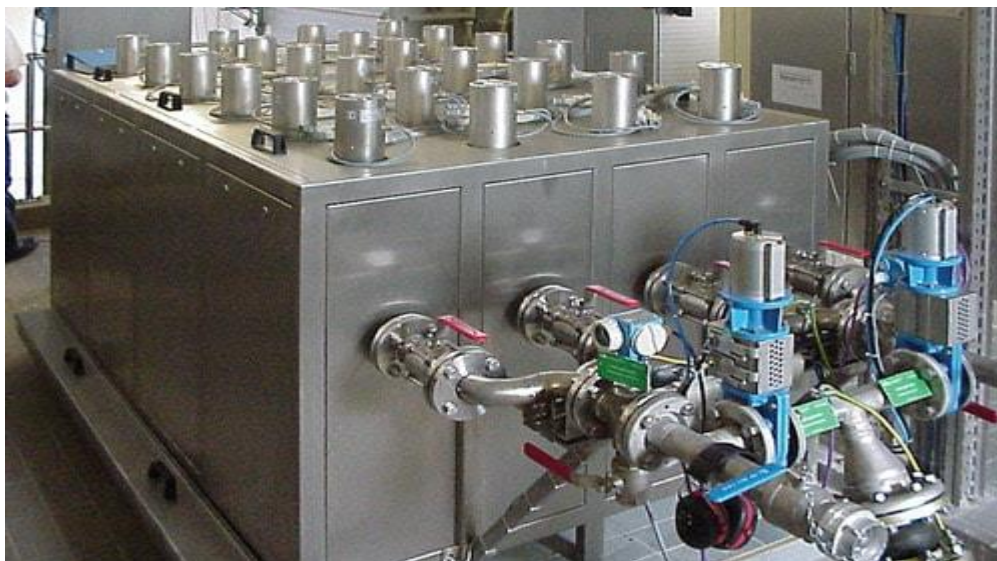
Figure 39: 48KW powerful ultrasonic processor for sludge disintegration
